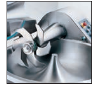
Standard removable 6 and 3-knife head
