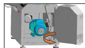
Large openings and folding electric distribution panel
