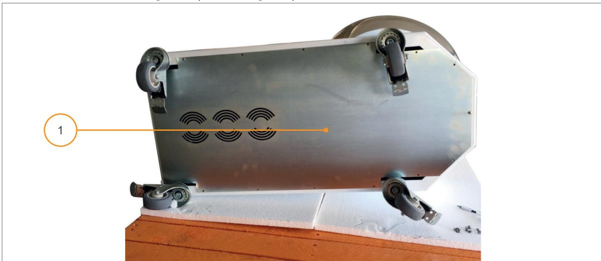
Fig. 8.7 - Bottom fixed guard removal
