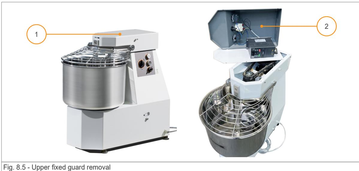
Fig. 8.5 - Upper fixed guard removal
