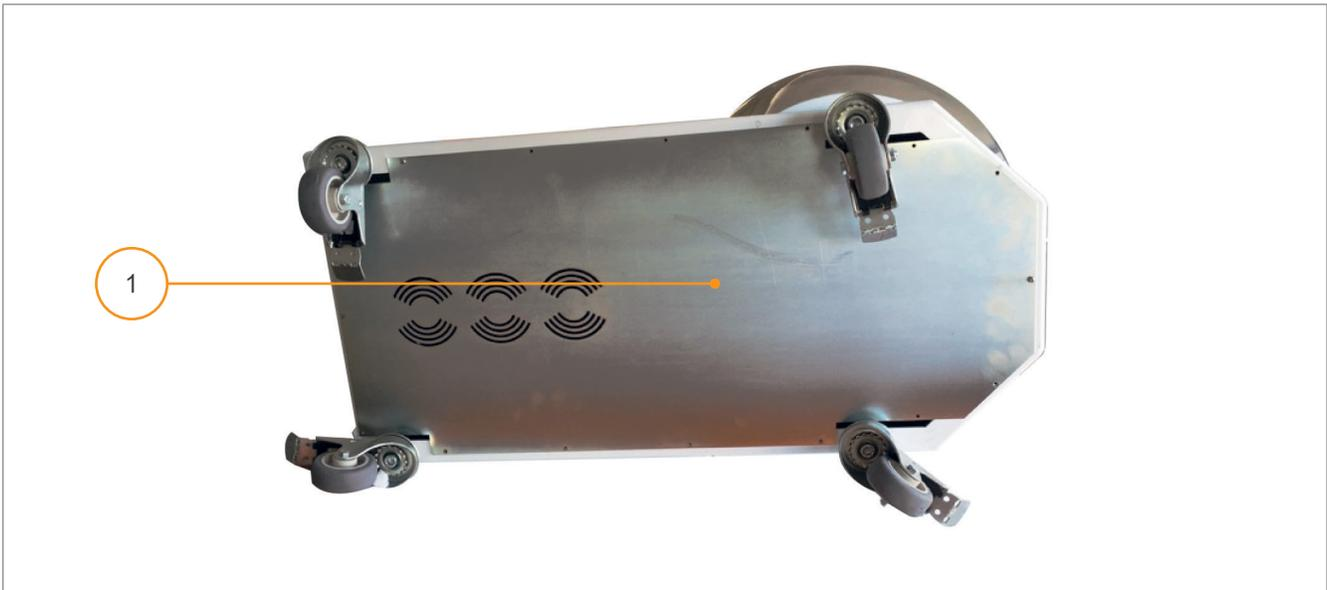
Fig. 8.3 - Rear fixed guard removal
