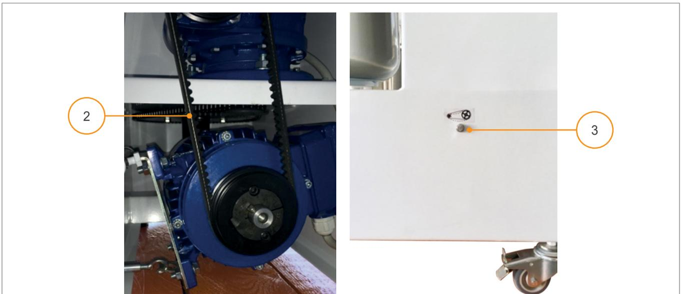
Fig. 8.2 - Tensioning the transmission belt
