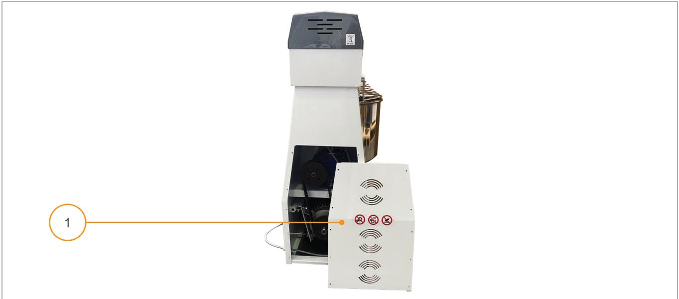
Fig. 8.1 - Rear fixed guard removal
