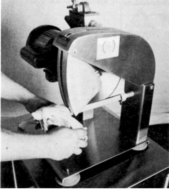
5. Drawing right drumstick and thigh with right hand down over apex of precision cutting guide bar, expose the location of the rump knuckle bone.
