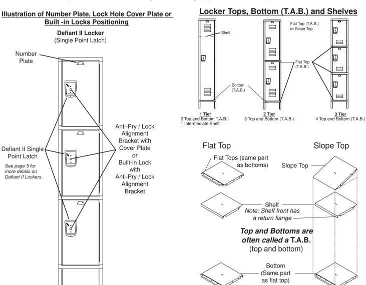
Single row lockers must be floor and wall anchored, double row lockers must be floor anchored and if possible wall or ceiling anchored.
