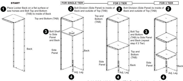
If legs are supplied, bolt Adjustable Leg inside of Side Panel (leg height can be adjusted to level and anchor locker)
