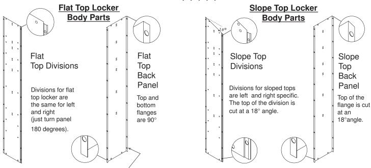
Bottom of divisons and back panels have the first hole on flange 1-3/4" from edge, (top of divisons and back panel have the first hole 1-1/4" from edge).
