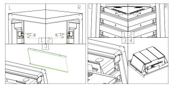
3. Remove the absorbent cotton. Take out the water tank assembly and update the absorbent cotton.
