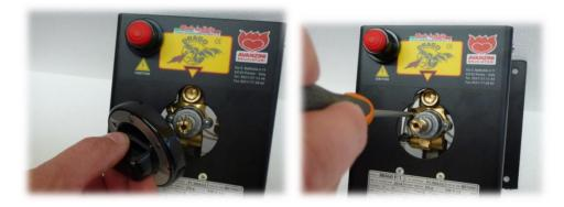
Insert again the handle. The low and high flame are now regulated, and with the handle it is possible to modify the heat requirements on the basis of what you are going to cook.
