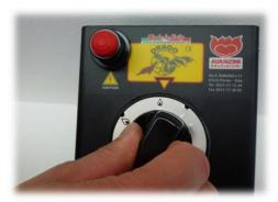
Extract the handle and regulate the high of the flame by acting on the screw (see images below). The right range is when the low flame length is about the half if compared to the long flame length. By turning it clockwise the gas power decreases, by turning it counter clockwise the gas power increases. (In any case when in low flame, the oven must not increase the temperature but maintain it).
