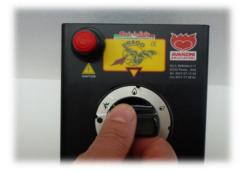
Extract the handle and regulate the height of the flame by acting on the screw (see images below). The right range is when the flame slightly overstep the centre of the oven's dome. By turning it clockwise the gas power decreases, by turning it counter clockwise the gas power increases.
