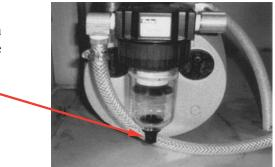
**MONTHLY:** The Part No. VTS529-1 filter element must be replaced once a month for proper vacuum and pump operation. Three (3) replacement filters have been included with your machine.
