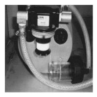
4. Separate the filter from the filter holders. Replace with a new filter.
