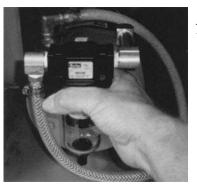
3. Unscrew the filter holder. Lower the filter carefully from the mounting stud. Note the order of parts.
