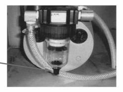
**MONTHLY:** The Part No. VTS529-1 filter element must be replaced once a month for proper vacuum and pump operation.
