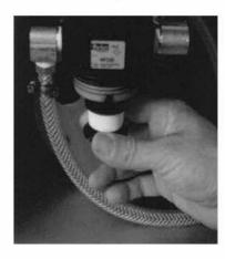
Separate the filter from the filter holders. Replace with a new filter.
